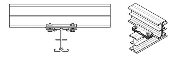
T84145 - Extension Bracket - WLL 100Kg - 350mm Drop T84150 - Extension Bracket - WLL 100Kg - 650mm Drop
