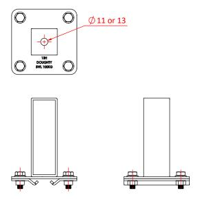
T84180 - 90° Rail to Tube Bracket - WLL 100Kg
