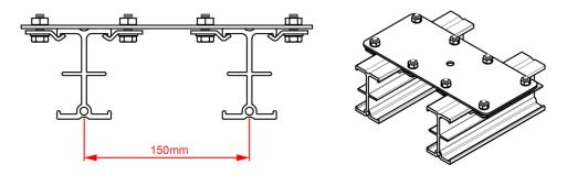
T84115 - Triple Spacer Plate - Not Suitable for Suspension
