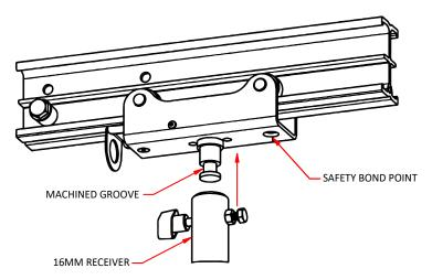
Carriages fitted with a 28mm spigot are designed to accept equipment fitted with a 28mm spigot. The receiver has three safety points incorporated into its design. The first point is a safety pin. This pin takes the initial weight of the equipment being suspended. The second point is the sword pin which secures the spigot in the receiver and still allows the spigot to rotate. The third point is the Doughty knob which stops the spigot rotating in the receiver.
