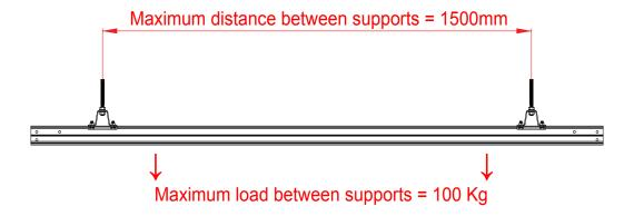
Studio Rail joints should be supported as illustrated. Unsupported joints must be treated as a pair of cantilevers.
