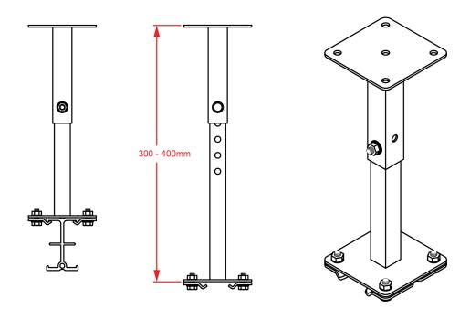
T84165 - Adjustable Angle Bracket - WLL 100Kg
