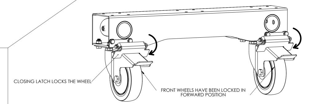
THE CASTER LOCKS ARE USED TO CONVERT A TROLLEY FROM A 4-WHEEL STEER TO A 2-WHEEL STEER CONFIGURATION. THIS LOCKS THE FRONT WHEELS, ALLOWING ONLY REAR WHEELS TO STEER FOR MORE CONTROL.
