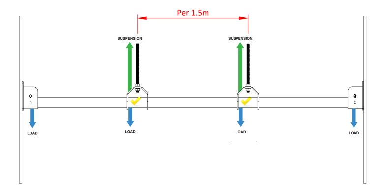
Example below shows a barrel grid using wall hangers and a combination of grid hangers.
