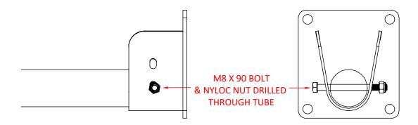
Standard Grid Hangers are folded steel hangers designed to suspend 48mm diameter tubes from an M12 stud or bolt fixing. They come in straight or corner variations. Ideal for suspending a barrel grid beneath aircon ducting etc. The hanger's width is the correct size to fit over many pipe clamp fittings.
